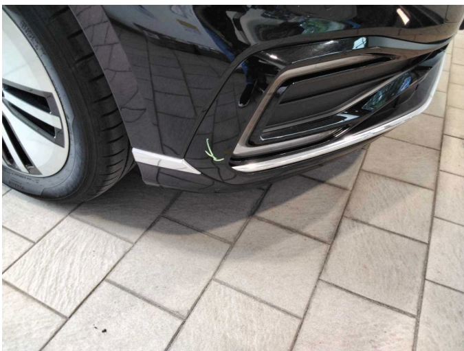
Damage 5: Front bumper: Front bumper - Scratch(es) - Paint
