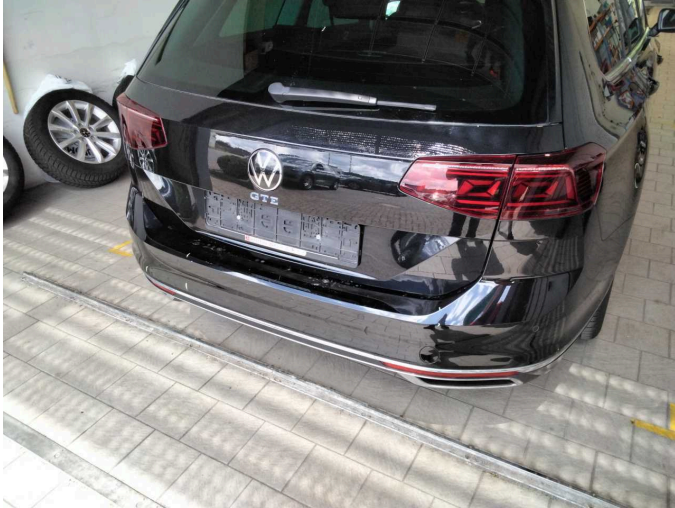
Damage 4: Rear bumper: Rear bumper - Scratch(es) - Paint
