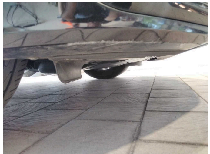
Damage 5: Front bumper: Front bumper - Scratch(es) - Paint
