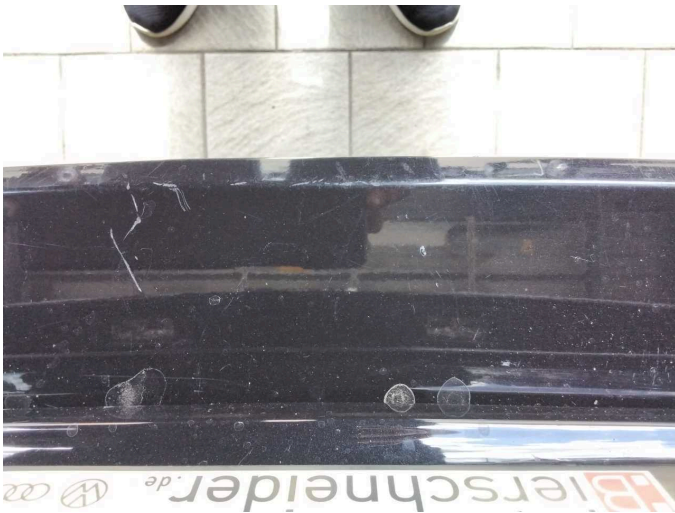
Damage 4: Rear bumper: Rear bumper - Scratch(es) - Paint
