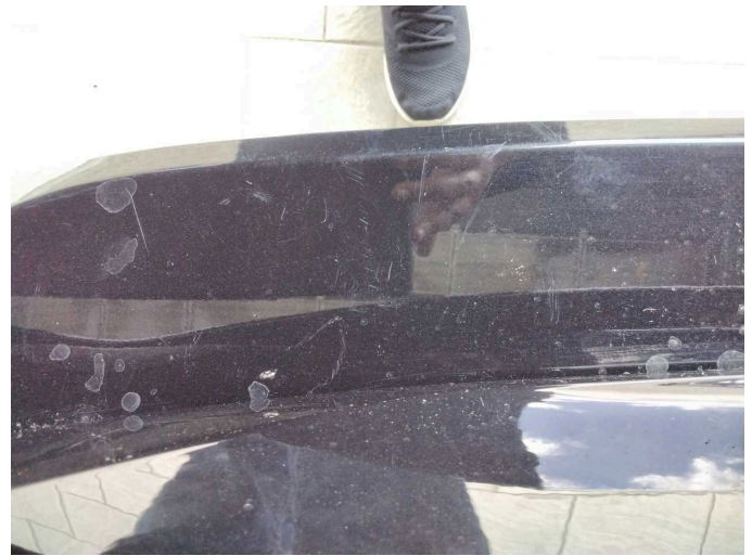
Damage 4: Rear bumper: Rear bumper - Scratch(es) - Paint
