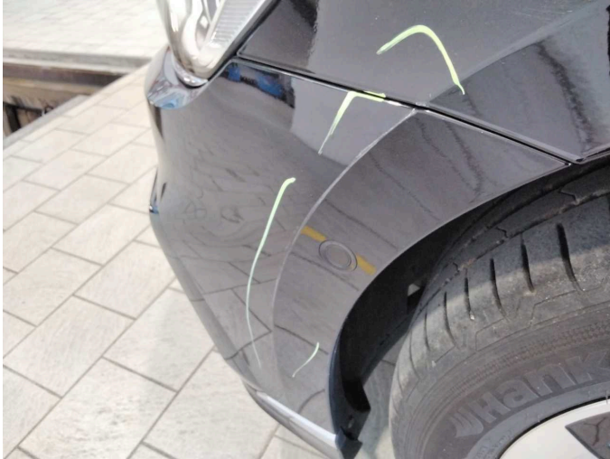
Damage 5: Front bumper: Front bumper - Scratch(es) - Paint
