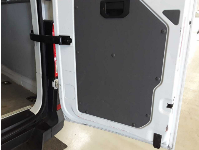
Damage 2: Boot lid / rear door: Trim washable - lower (rechts) - Broken / torn - Replace
