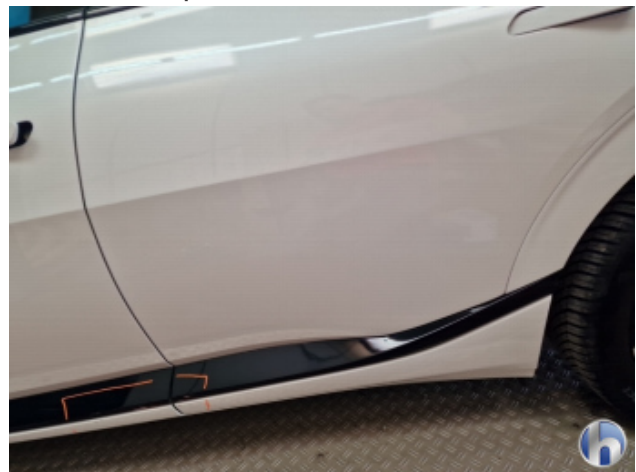
3. Tür Hinten - Links Kratzer - Smart Repair
