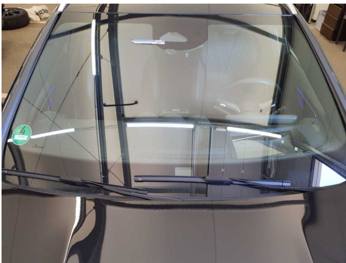
Damage 6: Vehicle glazing: Windscreen with lane departure assistant - Broken / torn - repair according to calculation
