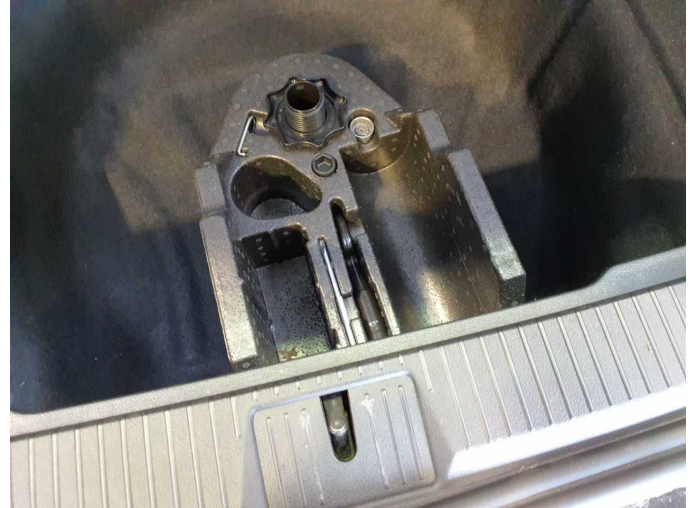
Missing part 1: Equipment: Tirefit compressor - Missing - Replace
