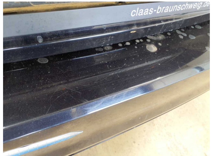
Damage 5: Rear bumper: Rear bumper - Dent / paintcoat damage - Paint
