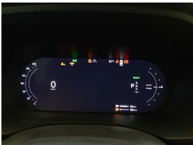
Damage 1: Instrument panel: Indicator light (Scheinwerfersystem) - Specify findings - Perform diagnosis
