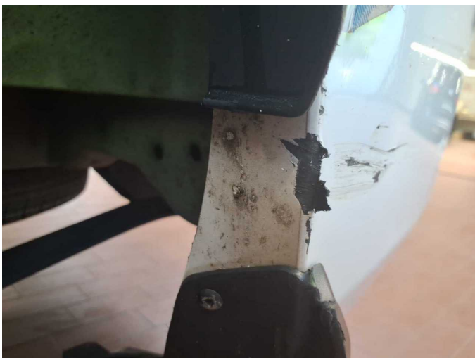
Damage 6: Rear bumper: Bumper - rear left side (+ Schmutzfänger verschürft erneuern) - Scratched - Repair and paint
