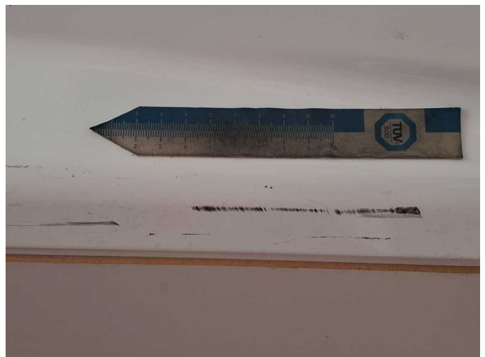
Damage 5: Boot lid / rear door: Boot lid - Dent / paintcoat damage - Loss in value
