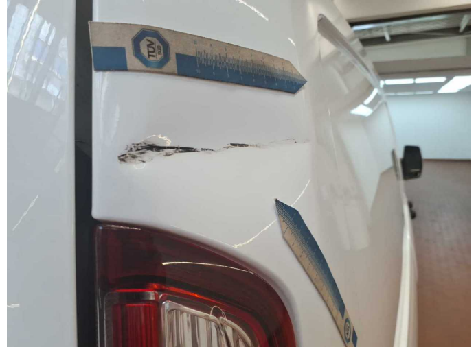
Damage 7: Body: D-pillar - right side - Dent / paintcoat damage - Repair and paint
