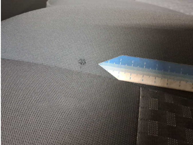
Damage 2: Seat - front: Seat cover - left side - Holes - Smart repair
