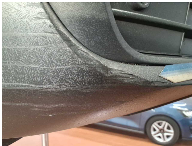
Damage 9: Front bumper: Spoiler - Scratched - Replace
