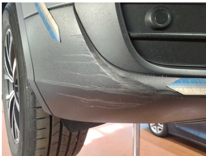
Damage 9: Front bumper: Spoiler - Scratched - Replace
