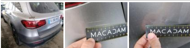
Tailgate / Boot, Dent(s), Repair and paint (complete)
