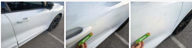
Door RR, Scratch(es), Repair and paint (complete)
