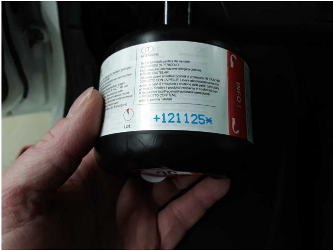
Damage 1: Equipment: Tirefit filler - Expired - Replace
