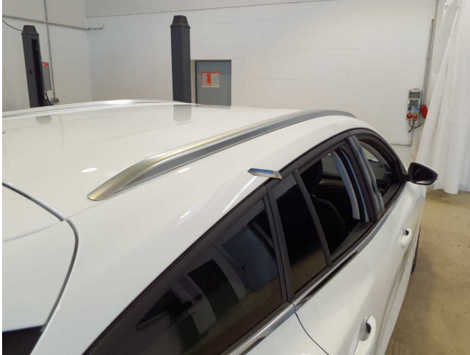
Damage 7: Roof: Roof rail - right side - dent(s) - Smart repair
