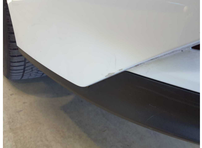
Damage 16: Rear bumper: Rear bumper - Scratch(es) - Paint
