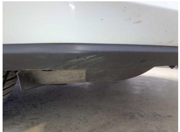
Damage 3: Front bumper: Spoiler - Scratch(es) - Replace
