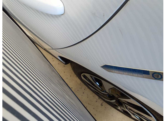
Damage 15: Side panel - rear left side: Side panel - Dent / paintcoat damage - Repair and paint
