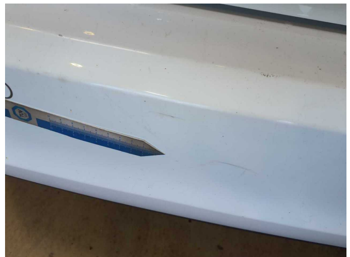
Damage 16: Rear bumper: Rear bumper - Scratch(es) - Paint
