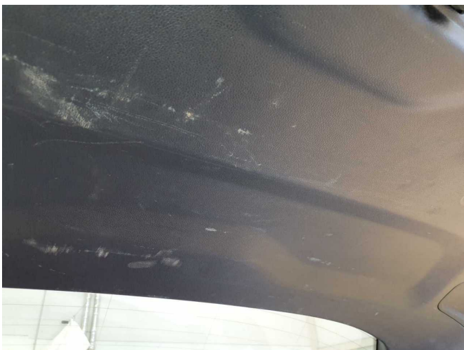
Damage 11: Trim / covers: Boot lid - interior trim - Scratch(es) - Replace
