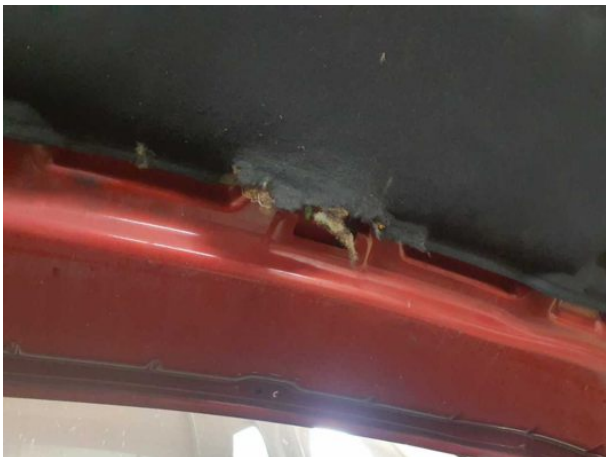
Damage #2: Bonnet: Insulation lining - Broken / torn - Replace
