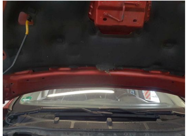
Damage #2: Bonnet: Insulation lining - Broken / torn - Replace
