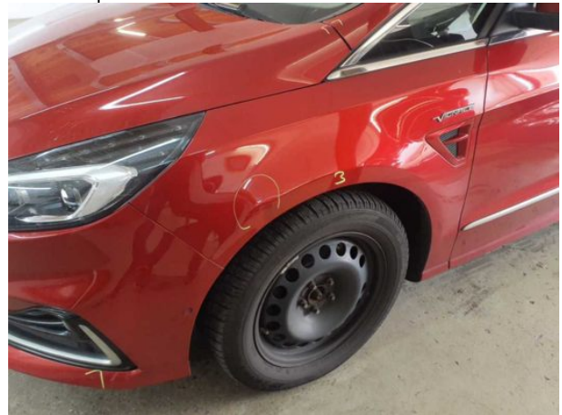
Damage #11: Mudguard - left side: Mudguard - left side - dent(s) - Repair and paint
