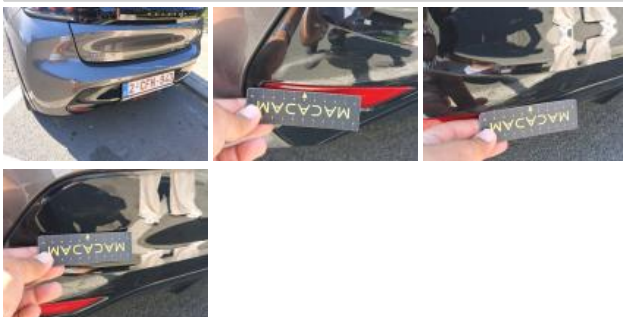
Bumper moulding R, Scratch(es), Repair and paint (complete)
