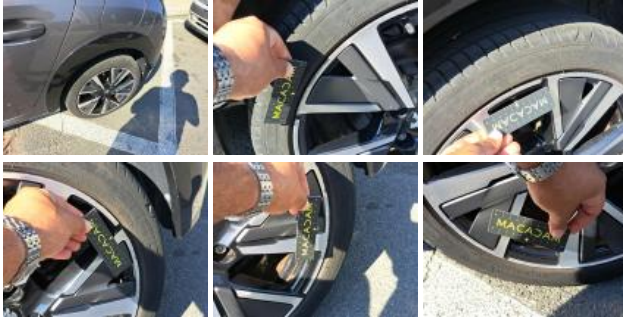
Tyre FL, Tear, Replace
