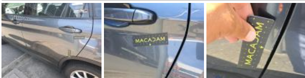
Door RL, Dent(s), Paintless dent repair
