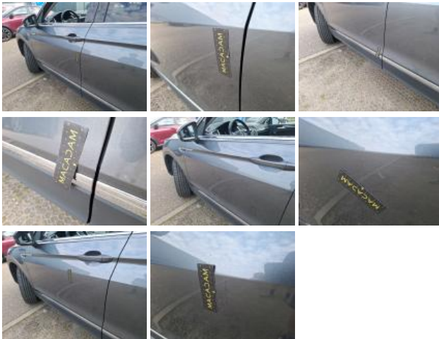
Door RL, Dent(s), Paintless dent repair
