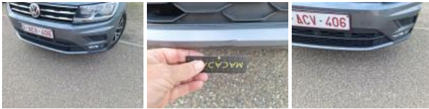
Bumper spoiler F, Scratch(es), Acceptable
