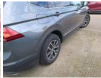
Wing RR, Dent(s) and scratch(es), Acceptable
