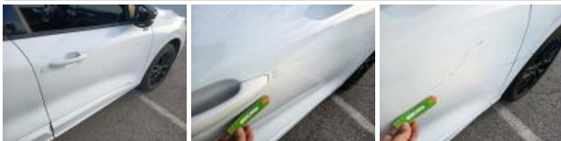
Door RR, Scratch(es), Repair and paint (complete)
