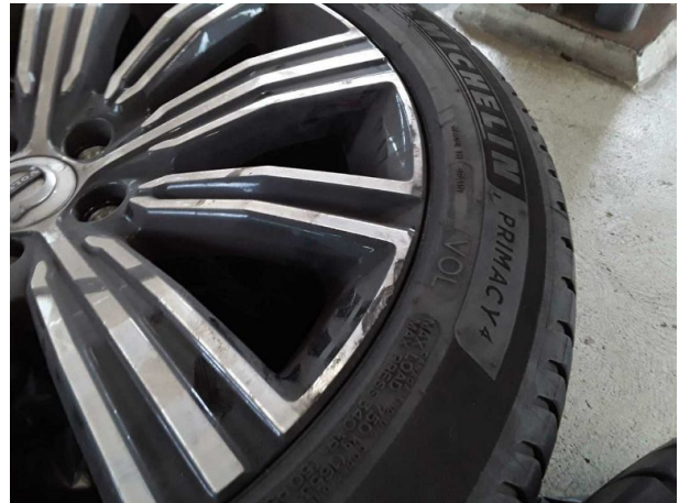
Damage #6: 2nd wheel set: Alloy rim set - complete - Scratch... - Loss in value
