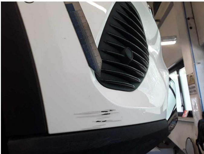
Damage 3: Front bumper: Front bumper - Scratched - Paint
