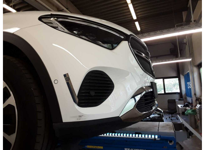
Damage 3: Front bumper: Front bumper - Scratched - Paint
