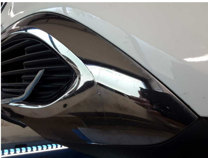
Damage 1: Front bumper: Spoiler - Broken / torn - Replace
