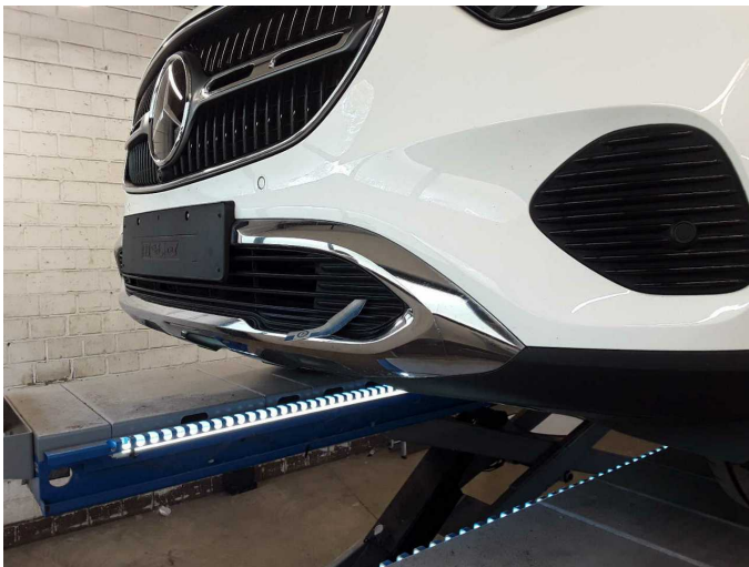
Damage 1: Front bumper: Spoiler - Broken / torn - Replace
