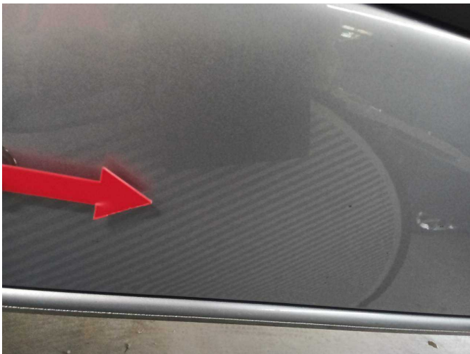
Damage 5: Sliding door, right: Sliding door - dent(s) - Smooth repair work
