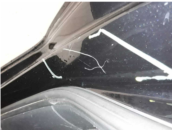
Damage #4: Side panel - rear right side: Sill - Scratched - Repair and paint
