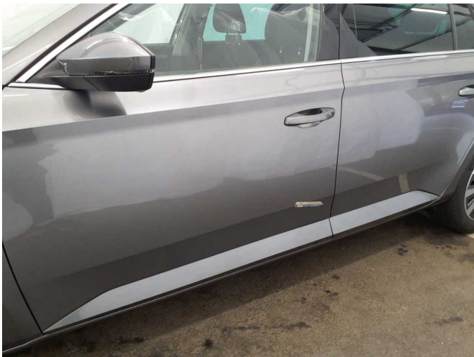
Damage 5: Door - front left side: Door - Dent / paintcoat damage - Smart repair
