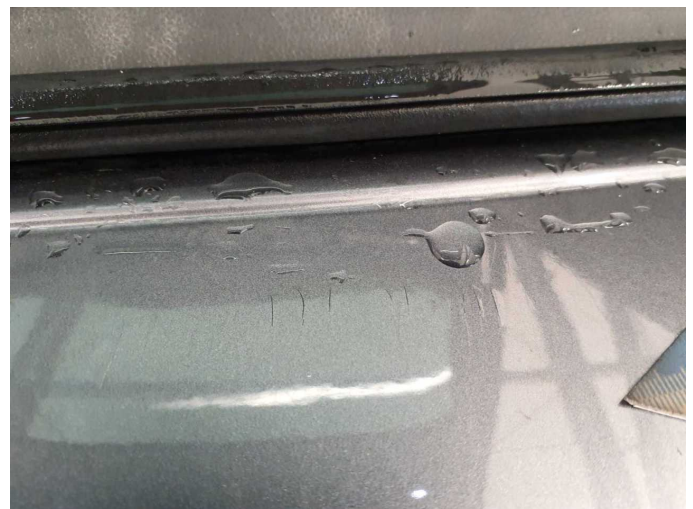
Damage 8: Rear bumper: Rear bumper (Lack ist rissig) - Paint defect - Paint
