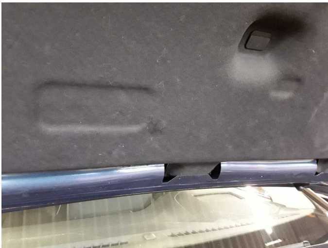
Damage 5: Bonnet: Insulation lining - Damaged - Replace
