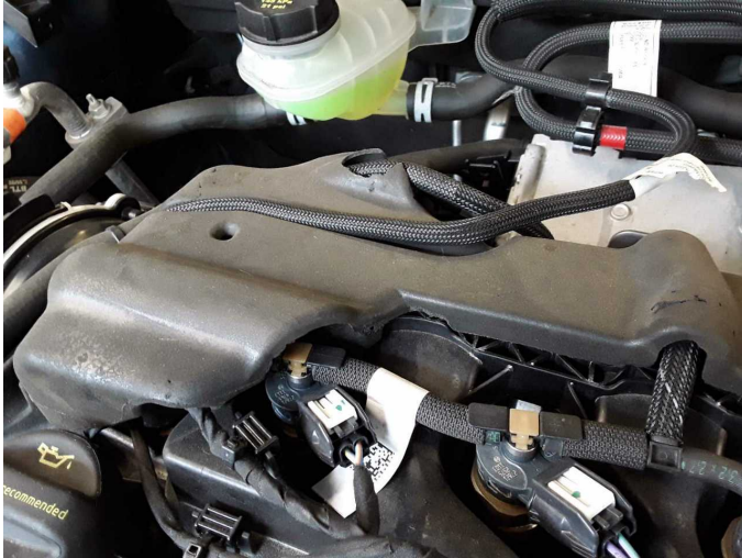
Damage 7: Engine: Engine cover - Damaged - Replace
