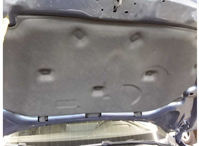
Damage 5: Bonnet: Insulation lining - Damaged - Replace
