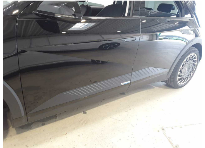
Damage 2: Door - front left side: Brightware - lower - Scratch(es) - Smart repair
