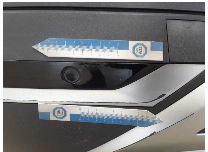
Damage 4: Rear bumper: Protection strip - left side - Scratch(es) - Smart repair
