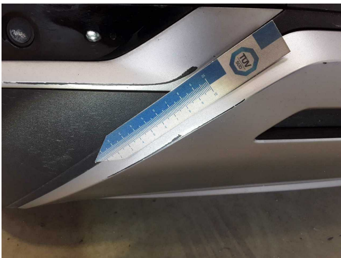
Damage 6: Rear bumper: Spoiler - Scratch(es) - Smart repair
