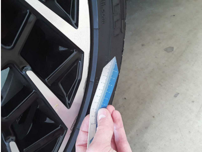
Damage 10: Wheel / tyres: Alloy rim - rear right side - Scratched - Replace
