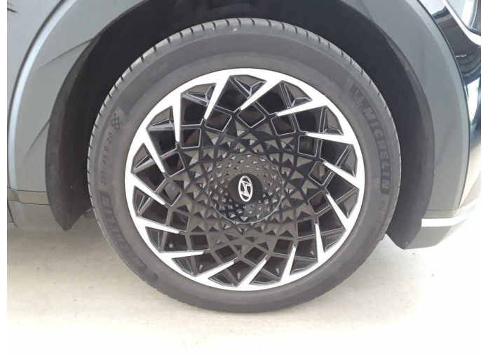
Damage 9: Wheel / tyres: Alloy rim - front right side - Scratch(es) - Loss in value
