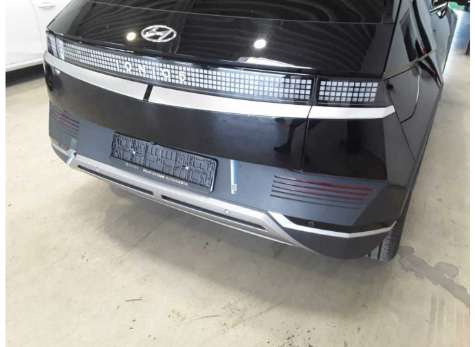
Damage 5: Rear bumper: Protection strip - centre - Scratch(es) - Smart repair
