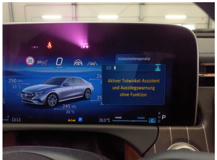
Damage 2: Instrument panel: Indicator light (Aktiver Totwinkel-Assistent) - Specify findings - Perform diagnosis
