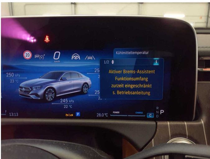
Damage 1: Instrument panel: Indicator light (Aktiver Brems-Assistent) - Specify findings - Perform diagnosis
