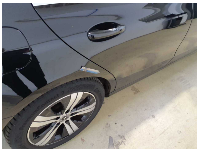
Damage 10: Side panel - rear right side: Side panel - Dent / paintcoat damage - Smart repair
