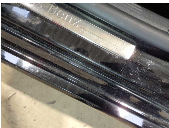
Damage 9: Sill - left side: Sill - Dent / paintcoat damage - Smart repair
