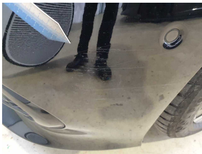
Damage 15: Front bumper: Front bumper (Inklusive anbauteile) - Scratched - Paint
