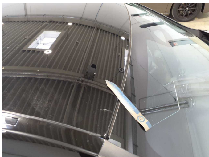
Damage 14: Roof: Roof - Scratch(es) - Paint
