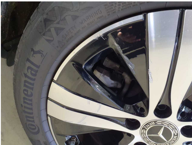
Damage 11: Wheel / tyres: Alloy rim - rear left side - Scratch(es) - Loss in value
