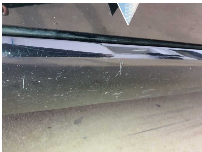
Damage 6: Sill - right side: Trim - Scratch(es) - Smart repair
