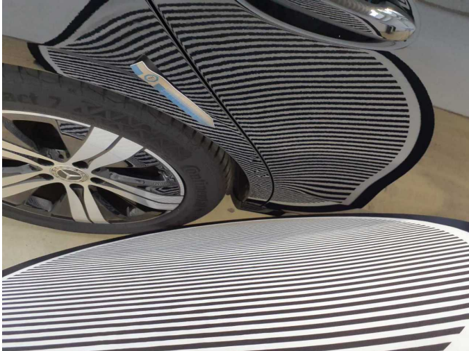
Damage 10: Side panel - rear right side: Side panel - Dent / paintcoat damage - Smart repair
