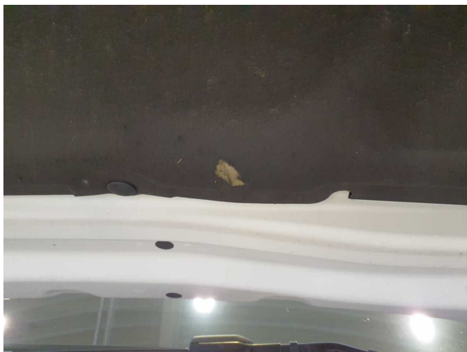
Damage 1: Bonnet: Insulation lining - Broken / torn - Replace
