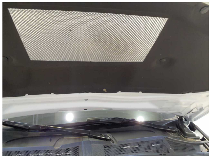
Damage 1: Bonnet: Insulation lining - Broken / torn - Replace
