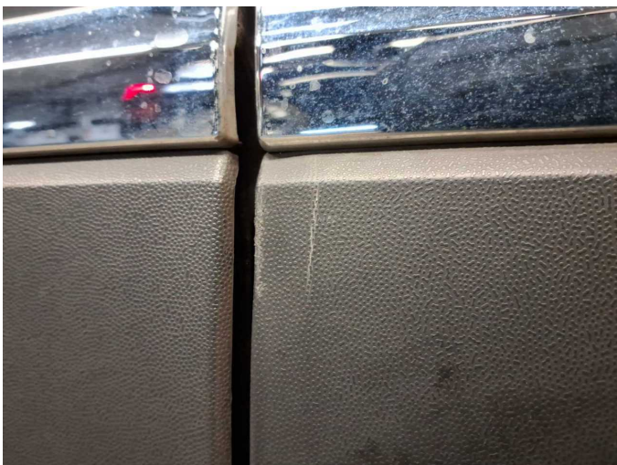
Damage 3: Door - front right side: Brightware - lower - Broken / torn - Replace
