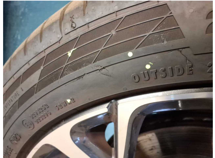
Damage 4: Wheel / tyres: Tyre - front right side (Flanke) - Damaged - Replace
