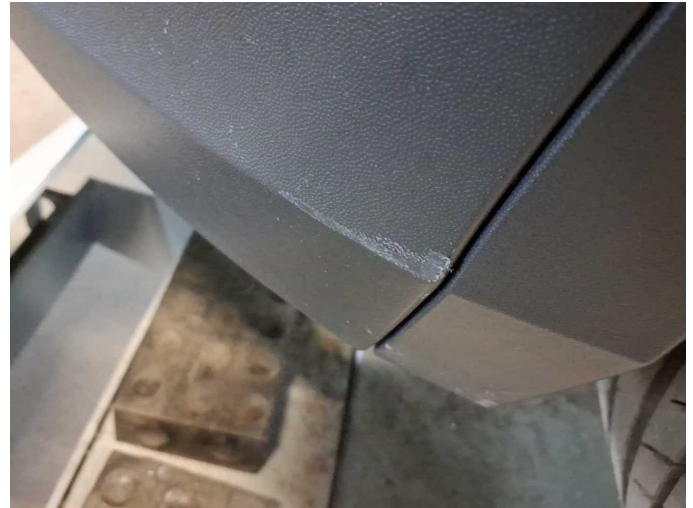
Damage 2: Front bumper: Spoiler - Scratch(es) - Smart repair
