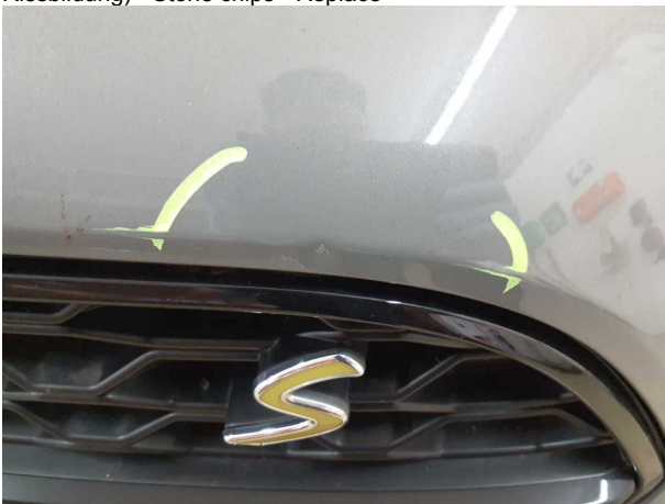
Damage #6: Bonnet: Bonnet - Dent / paintcoat damage - Repair and paint
