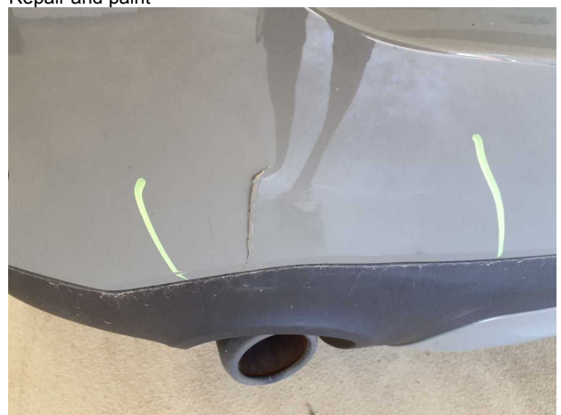
Damage #7: Rear bumper: Rear bumper - Damaged - Replace
