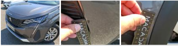
Roof pillar R, Dent(s), Acceptable
