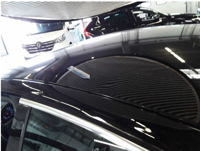
Damage 2: Roof: Roof - dent(s) - Smooth repair work
