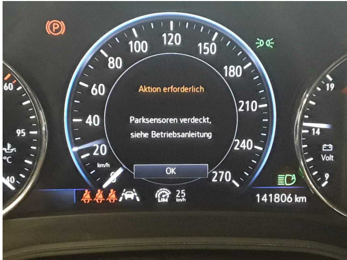
Damage 3: Front bumper: Parking sensors - centre - Electrical fault - Perform diagnosis
