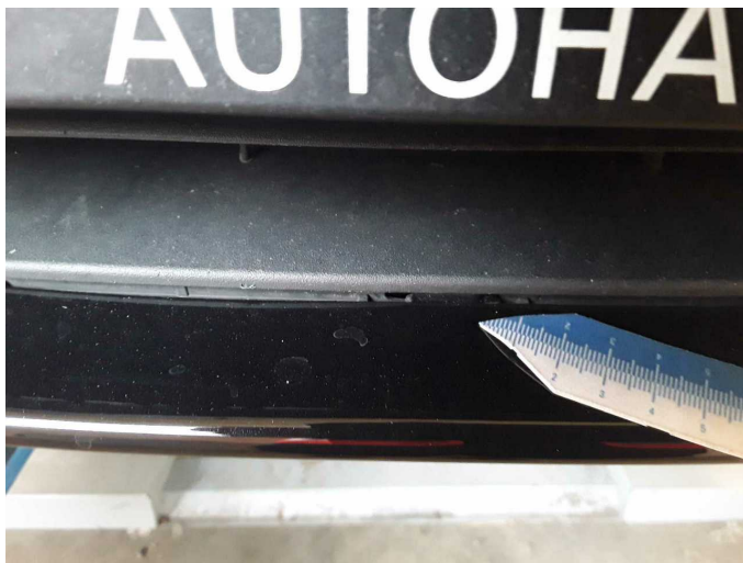
Damage 4: Front bumper: Air-inlet grille - Malposition - Set / adjust
