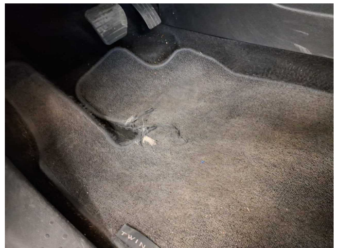
Damage 1: Trim / covers: Floor mats - Damaged - Replace
