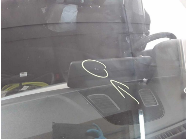
Damage #11: Vehicle glazing: Windscreen (Rissbildung) - Stone chips - Replace
