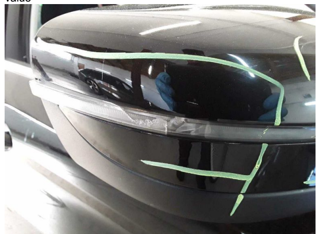
Damage #7: Indicator - front: Mirror - right side - Damaged - Replace
