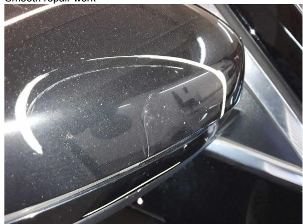
Damage #10: Wing mirror - right side: Cap (Gebrochen) - Damaged - Replace
