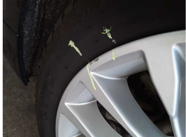
Damage #3: Wheel / tyres: Alloy rim - rear left side - Scratched - No deduction
