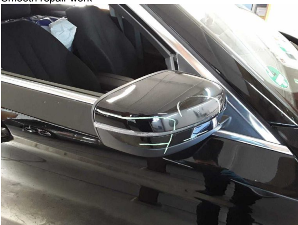
Damage #10: Wing mirror - right side: Cap (Gebrochen) - Damag... - Replace
