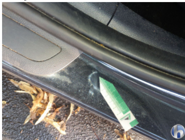
1. Schweller - Links Kratzer - Smart Repair
