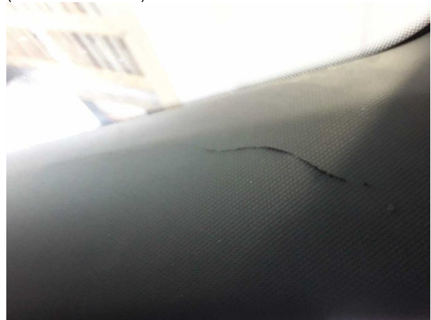
Damage #10: Trim / covers: Trim / covers (A Säule) - Scratch... - Replace
