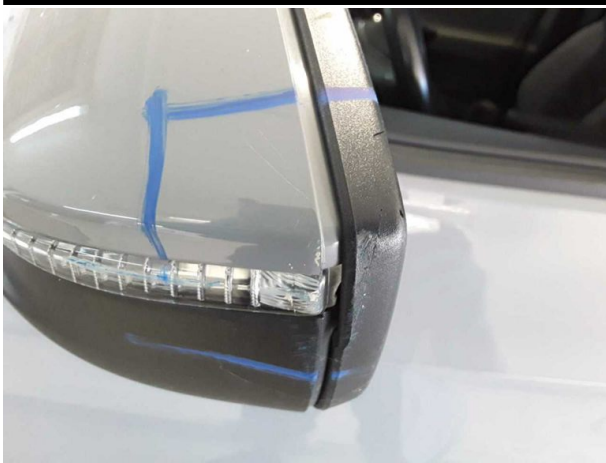
Damage #12: Wing mirror - left side: Cap - Scratched - Smart repair
