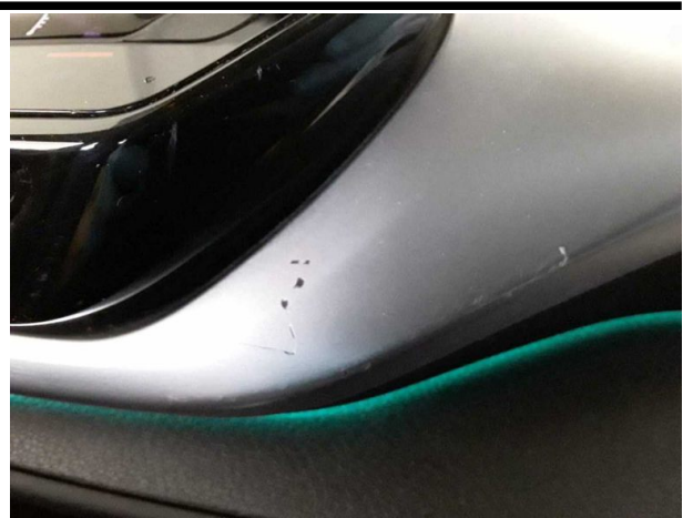
Damage #9: Trim / covers: Brightware / decorative strip (Mittelkonsole vorne) - Scratched - Loss in value
