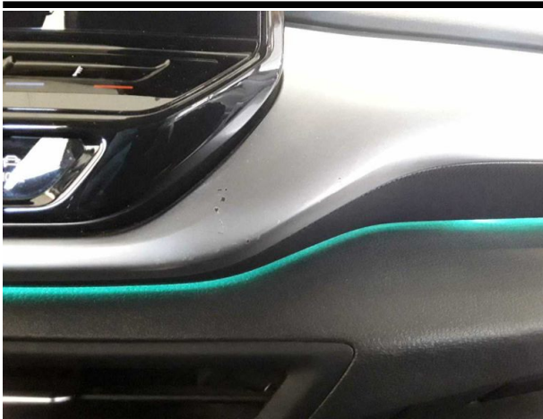
Damage #9: Trim / covers: Brightware / decorative strip (Mittelkonsole vorne) - Scratched - Loss in value
