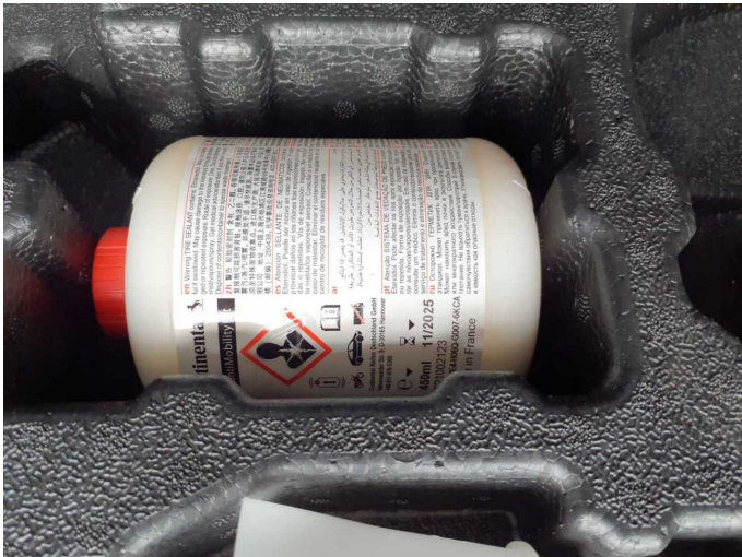
Damage 1: Equipment: Tirefit filler - Expired - Replace
