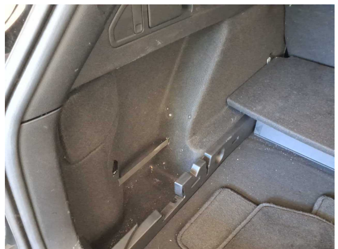
Damage 10: Trim / covers: Cargo area - lining -left side (Fehlbohrungen) - Differs from the original configuration - Replace
