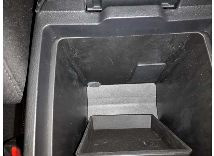
Damage 3: Interior: Arm rest, front (Deckel hinten, Fehlbohrungen) - Differs from the original configuration - Replace
