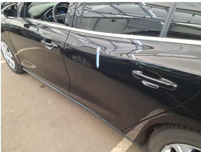
Damage 14: Door - rear left side: Door - Scratched - Paint
