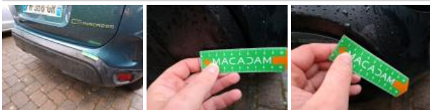
Bumper R, Scratch(es), Repair and paint (complete)
