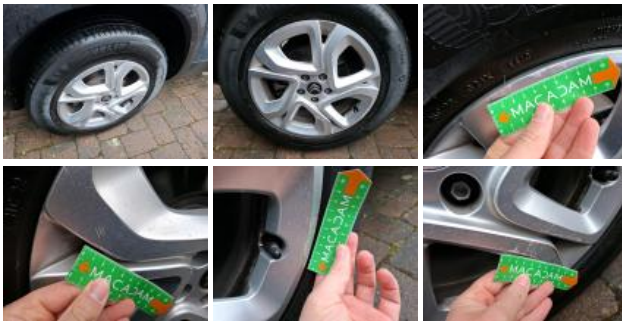
Tyre FR, Out of tolerance, Replace
