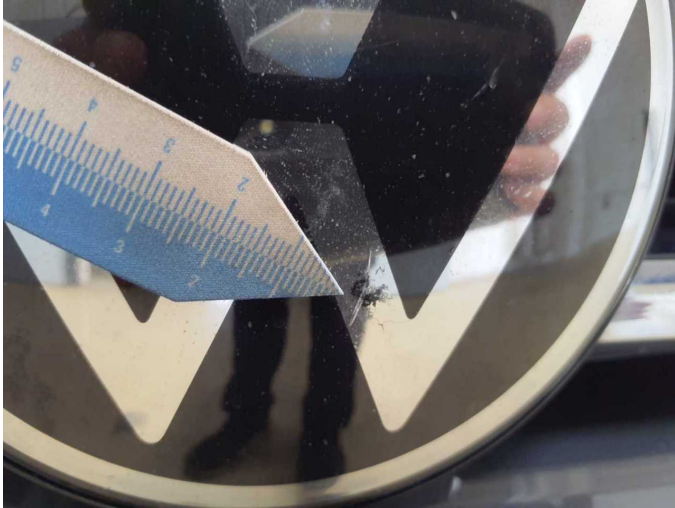
Damage 8: Bonnet: Emblem - Broken / torn - Replace
