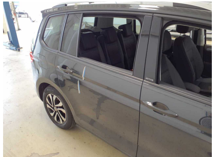
Damage 9: Door - rear right side: Door (Anätzung) - Paint defect - Repair and paint
