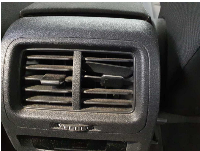
Damage 7: Instrument panel: Air nozzle - centre (Hinten) - Broken / torn - Replace
