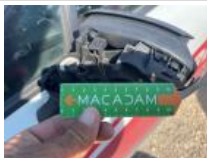
Outside rear-view mirror housing L, Missing, Replace and paint
