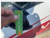
Outer sill L, Dent(s) and scratch(es), Repair and paint (complete)
