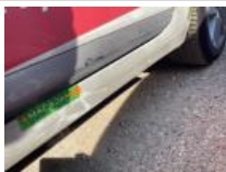
Outer sill L, Dent(s) and scratch(es), Repair and paint (complete)
