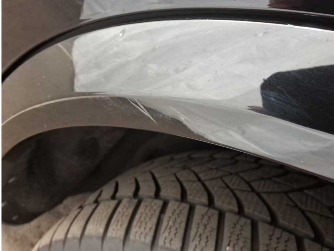
Damage 4: Side panel - rear left side: Wheel well extension - Scratch(es) - Smart repair
