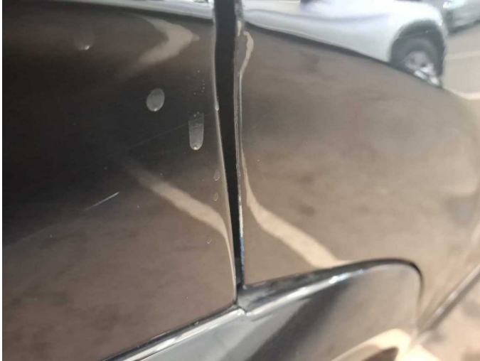
Damage 10: Door - rear right side: Door - Dent / paintcoat damage - Paint
