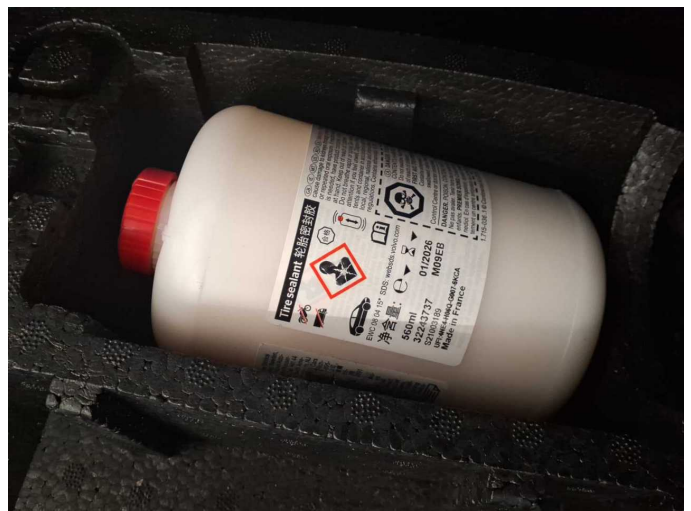
Damage 1: Equipment: Tirefit filler - Expired - Replace
