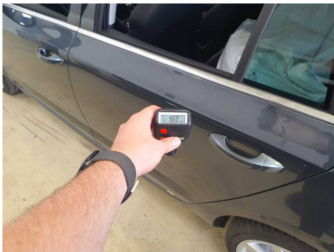
Repainting 2: Door - rear left side
