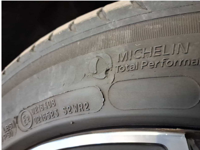
Damage 5: Wheel / tyres: Tyre - front left side (Flanke) - Damaged - Replace
