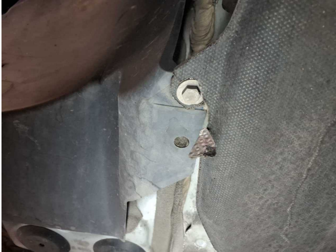
Damage 12: Engine: Engine cowling - lower - Broken / torn - Replace
