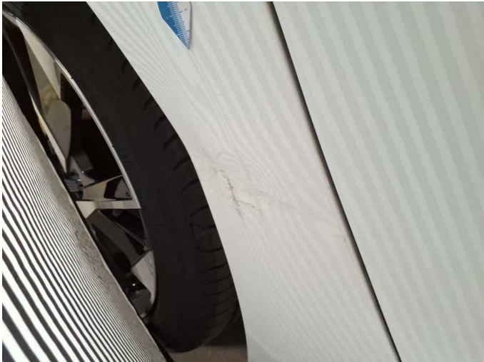
Damage 16: Side panel - rear right side: Side panel - Deformed - Repair and paint
