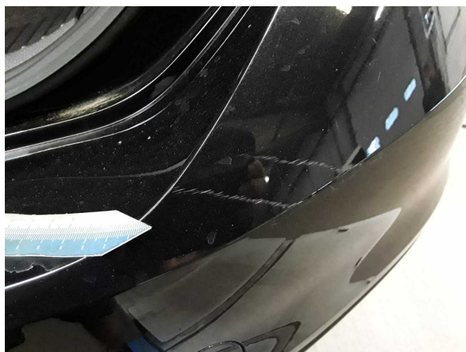
Damage 8: Rear bumper: Rear bumper - Scratch(es) - Paint
