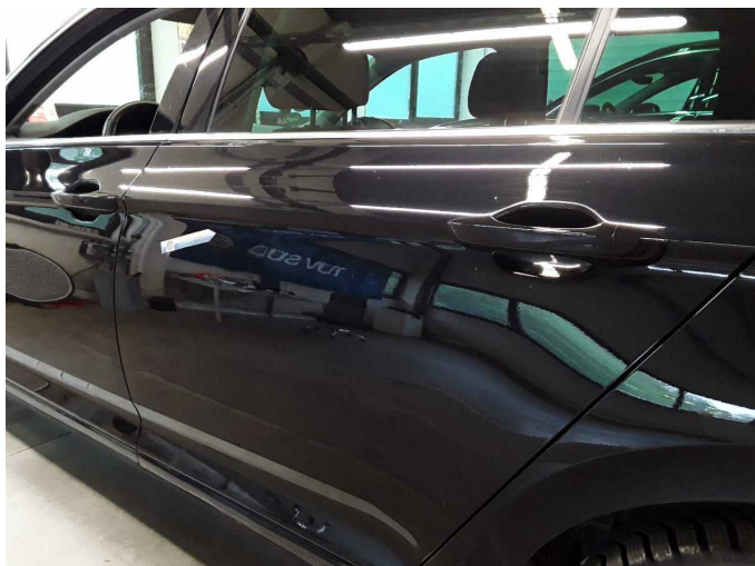
Damage 9: Door - rear left side: Door - Deformed - Repair and paint
