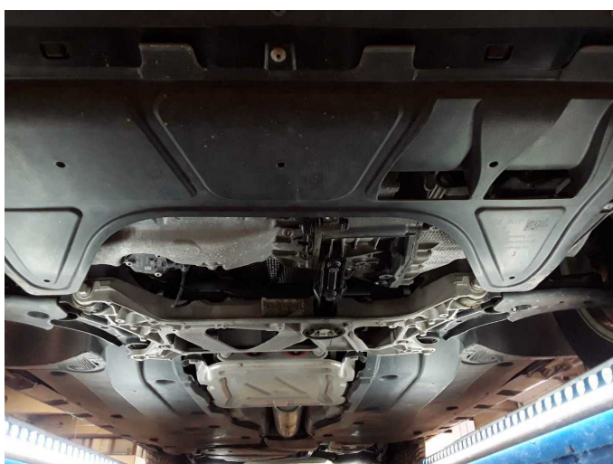
Damage 6: Body: Underbody panelling - Missing - Replace
