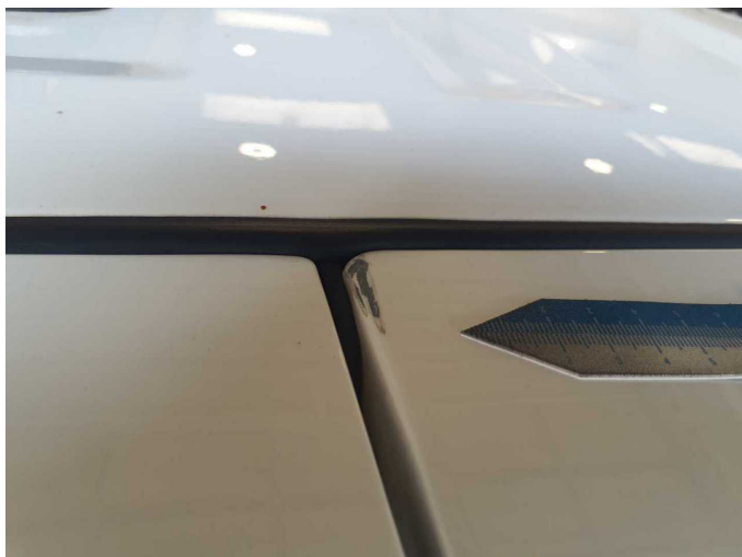
Damage 4: Boot lid / rear door: Rear door - right side - Scratch(es) - Smart repair
