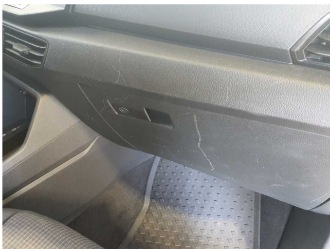
Damage 3: Instrument panel: Centre console - front - Scratch(es) - Loss in value
