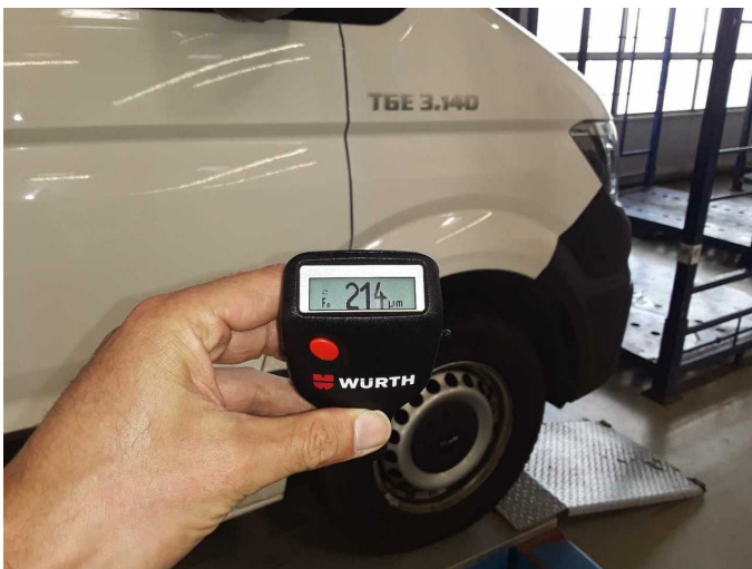
Mudguard - right side: 214 µm
