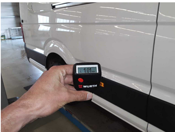
Side panel - rear right side: 1,010 µm
