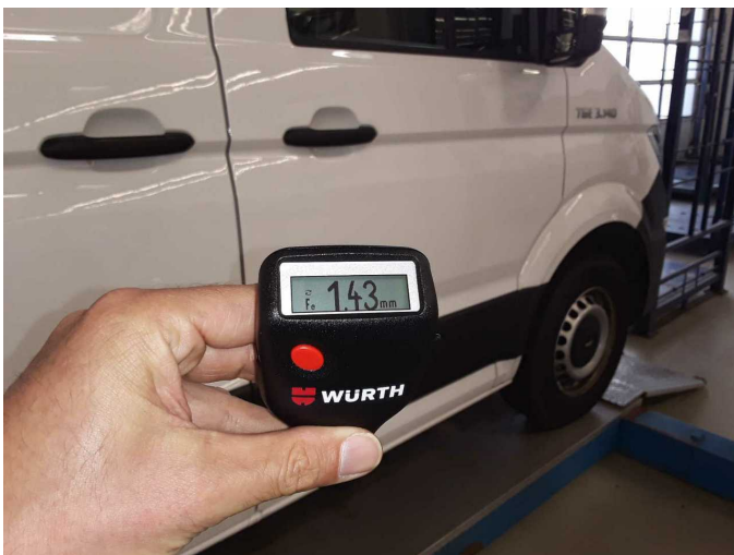
Door - front right side: 1,430 µm
