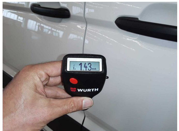
Door - front right side: 1,430 µm
