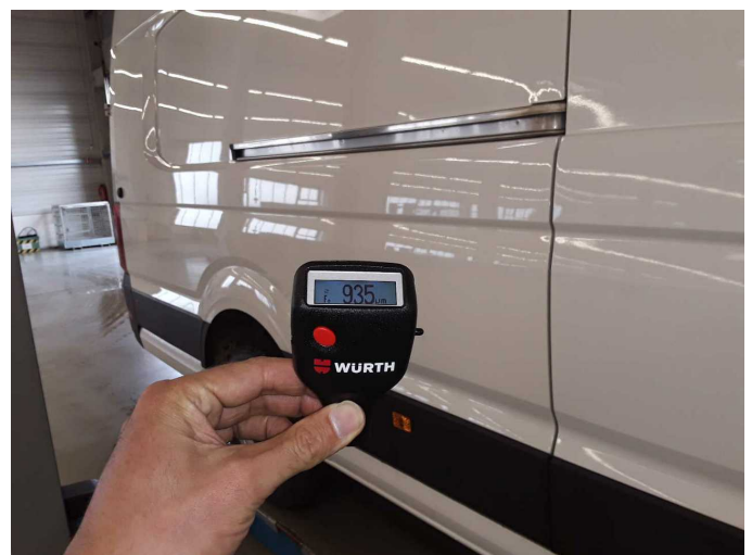
Side panel - rear right side: 1,010 µm
