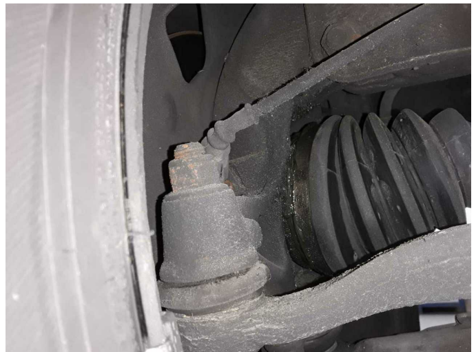
Damage 1: Drive train: Sleeve prop shaft - front left side - Leaking - Replace
