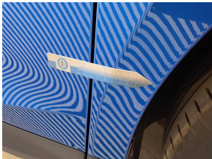
Damage 3: Mudguard - right side: Mudguard - right side - Deformed - Repair and paint
