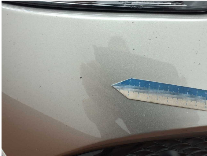
Damage 7: Front bumper: Front bumper (Steinschläge) - Scratched - Paint
