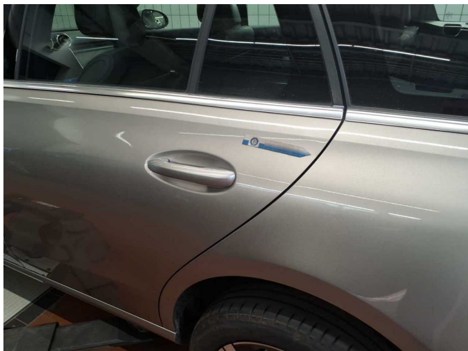
Damage 2: Door - rear left side: Door edge - Dent / paintcoat damage - Smart repair
