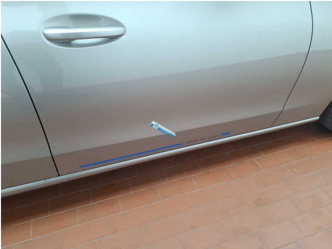
Damage 1: Body: Body - Glued / labelled - De-glue / neutralise
