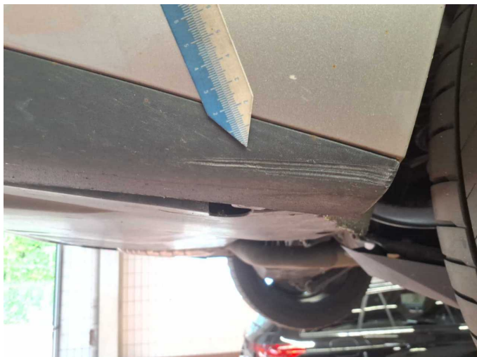
Damage 5: Rear bumper: Spoiler - Scratch(es) - Replace
