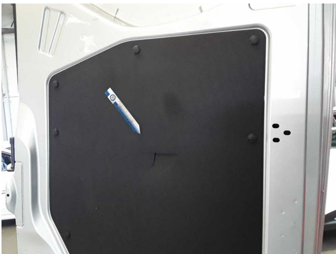
Damage 3: Trim / covers: Boot lid - interior trim - Damaged - Replace
