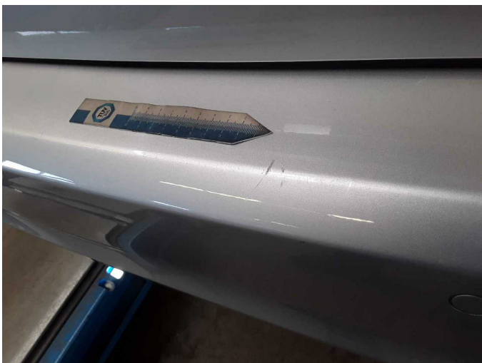
Damage 3: Rear bumper: Rear bumper - Scratch(es) - Paint
