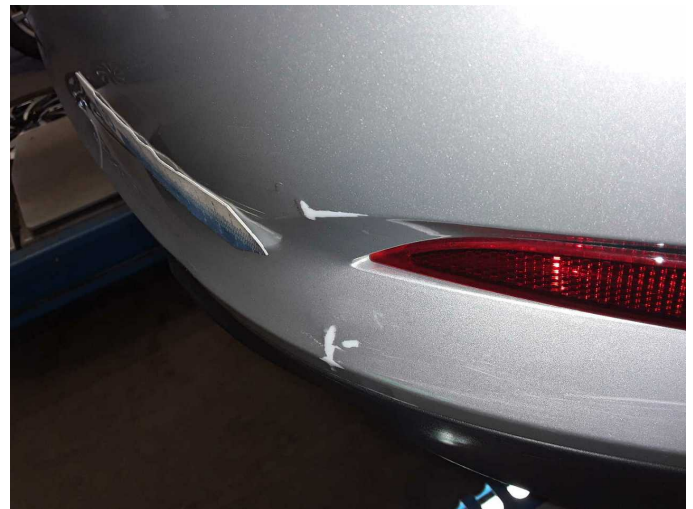
Damage 3: Rear bumper: Rear bumper - Scratch(es) - Paint
