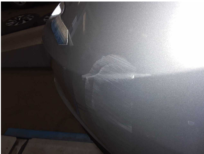
Damage 3: Rear bumper: Rear bumper - Scratch(es) - Paint
