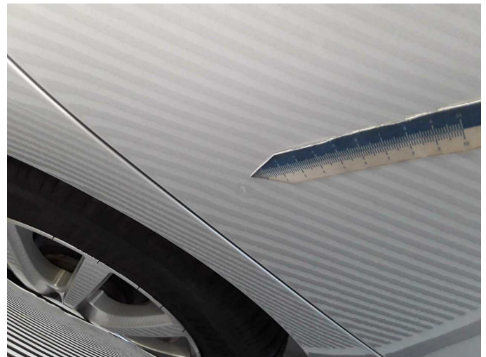
Damage 6: Door - rear right side: Door - Dent / paintcoat damage - Repair and paint
